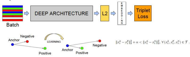
$$\text{Triplet Loss function: } \sum_{i}^{N} \left[ \|f(x_i^a) - f(x_i^p)\|_2^2 - \|f(x_i^a) - f(x_i^n)\|_2^2 + \alpha \right]_+ \\ \qquad \text{Where } f \text{ is the embedding }$$
